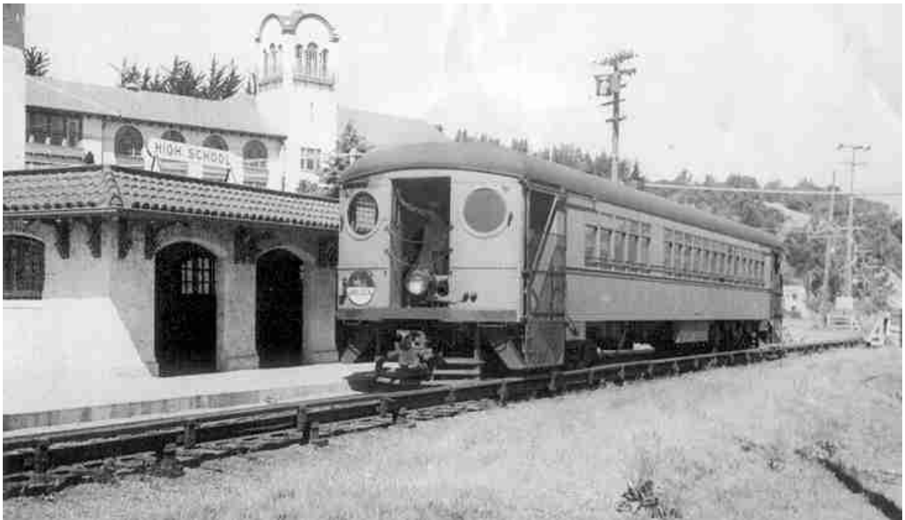
NWP electric passenger motor 383 at High School Station near Mill Valley, July 1937. St. Louis Car Co. 1930. Electric 3rd rail this side of car. Mill Valley Branch electric trains quit on 9/30/40 and the entire NWP interurban system serving San Rafael, San Anselmo and Manor was abandoned 2/28/41.
